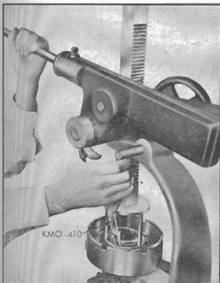
Fig. 24 Removing clutch spring snap ring. 1950-52
